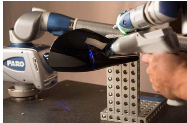
Figure 1.1. 3D Laser Scanner Working
